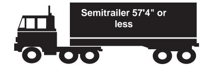
No overall length limit for a combination with a single trailer length of **57' 4" (14.47 meters)** or less in length. **C.R.S. 42-4-504(4)**
