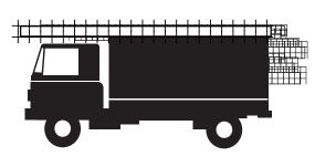
Load may not project more than **10** feet **(3.05 meters)** to the rear of the vehicle bumper. Overhangs for automobile and boat transporters are restricted to **6** feet **(1.83 meters)**. **C.R.S. 42-4-504(6)**
