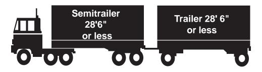
No overall length limit for a combination of units with trailers **28'6" (8.68 meters)** or less in length. The common name for this combination is "Western Double".
