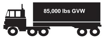
Maximum gross weight allowed on any Colorado noninterstate highway is **85,000 pounds (38,556 kg).** In addition vehicles must comply with the axle weight limitations and the Colorado Bridge Formula. **C.R.S. 42-4-508(1)(b)**
