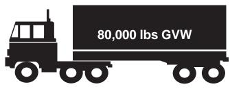
Maximum gross weight allowed on any Colorado Interstate highway is **80,000 pounds (36,288 kg).** In addition vehicles traveling on interstate highways must comply with the Federal Bridge Formula. **C.R.S. 42-4-508 (1)(c)(III)**
