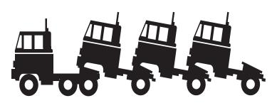
Saddlemounts are allowed **75'** (**22.86 meters**) in length for no more than **4** total units. A fullmount also may be transported as part of this combination. A fullmount is a smaller vehicle that is mounted completely on the frame of either the first or last vehicle in a saddlemount combination. **C.R.S. 42-4-504(4.5)**
